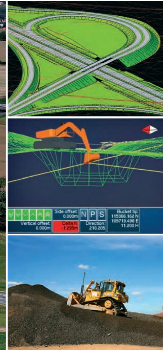
A1 motorway, Gdańsk – Toruń is the largest single-road construction project in Europe as far as equipment used is concerned. The project itself is unique because it facilitates BIM technology and 3-D GPS systems, which allow Skanska to complete and deliver the highest quality project a full year ahead of schedule.
