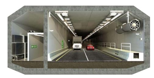
Reflecting the input provided by local police, fire, ambulance and first responders, the design will enable enhanced emergency response and evacuation readiness. State-of-the-art safety features in the new tunnel include a separate escape corridor, jet fans, deluge system, fire sensors, fire alarms/extinguishers/hose connections, motorist aid phones, fireproofing and video monitoring for traveler safety.
